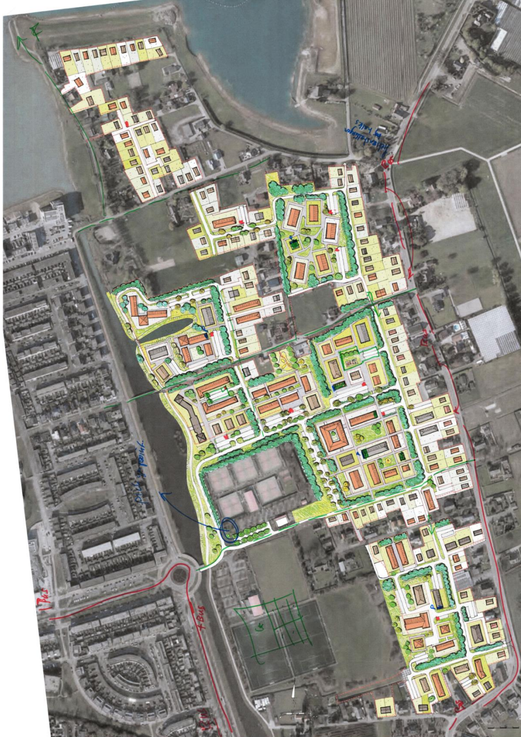
Figure 14: Various transport modes drawn on the draft of Vossenpels-Noord with bus connections (red lines), pick-up delivery point (blue circle in southwest corner), central parking locations (green square in the middle), shared cars (spread red squares) and bicycle sheds combined with shared facilities (green blocks as parts of the buildings)
